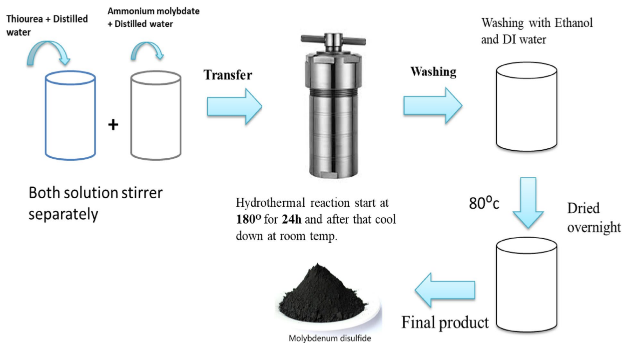
Figure 9: Schematic diagram of hydrothermal method for the synthesis of MoS 2 .
