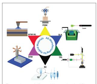
Figure 5. A survey of different additive manufacturing (AD) technologies that can be adapted in the fabrication of hybrid materials: fused deposition modeling (FDM), stereolithography (SLA), two-photon lithography (TPL), reactive extrusion (RE), direct ink writing (DIW), and atomic force microscopy-based nanolithography (AFM-NL).
