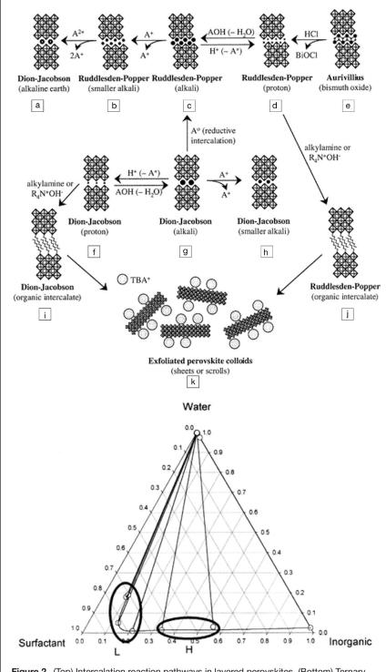
Figure 2. (Top) Intercalation reaction pathways in layered perovskites. (Bottom) Ternary phase diagram for lamellar (L) versus hexagonal (H) liquid-crystal formation from Reference 9. (Top) Adapted with permission from Reference 8. © 2002 American Chemical Society. (Bottom) Adapted with permission from Reference 9. © 2002 American Chemical Society.
