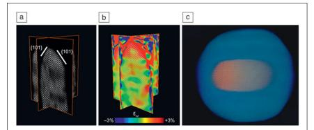
**Figure 2.** (a) Slices through a 3D reconstruction of an Au nanorod showing the atomic lattice. (b) Corresponding slices through the strain field along the major axis of the nanorod, indicating an outward relaxation at the tip of the nanorod. (c) 3D visualization of a core–shell Au@Ag nanorod, where the Au core is rendered orange, and the Ag atoms are visualized in blue.<sup>20,22</sup>
