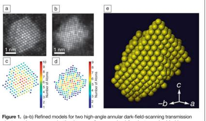
electron microscope projection images of a nano-sized Ag cluster embedded in an Al matrix. (c–d) Number of Ag atoms per projected atomic column for both images. (e) 3D reconstruction of the Ag nanoparticle, based on discrete tomography.<sup>12</sup>
