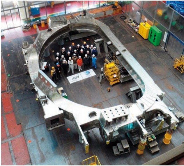
Figure 10. Casing of a toroidal field coil for ITER (courtesy: ITER Organization; more photos on component production available under: https://www.iter.org/album/Media/2%20-%20Manufacturing%20underway ).
