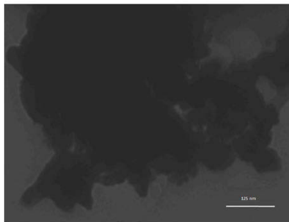
FIG. 1. (a) XRD profile of the pure ZnS and ZnS(Ag) nanoparticles with and without annealing at 950 °C in a vacuum. (b) TEM micrograph of the as synthesized ZnS(Ag) powder.
