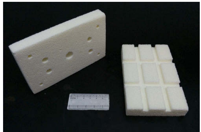
FIG. 10. Photograph of alumina foam bodies prepared by carbon burnout and sintering of green machined carbon bonded alumina foam bodies. The slots are made by milling and holes are made by drilling.
