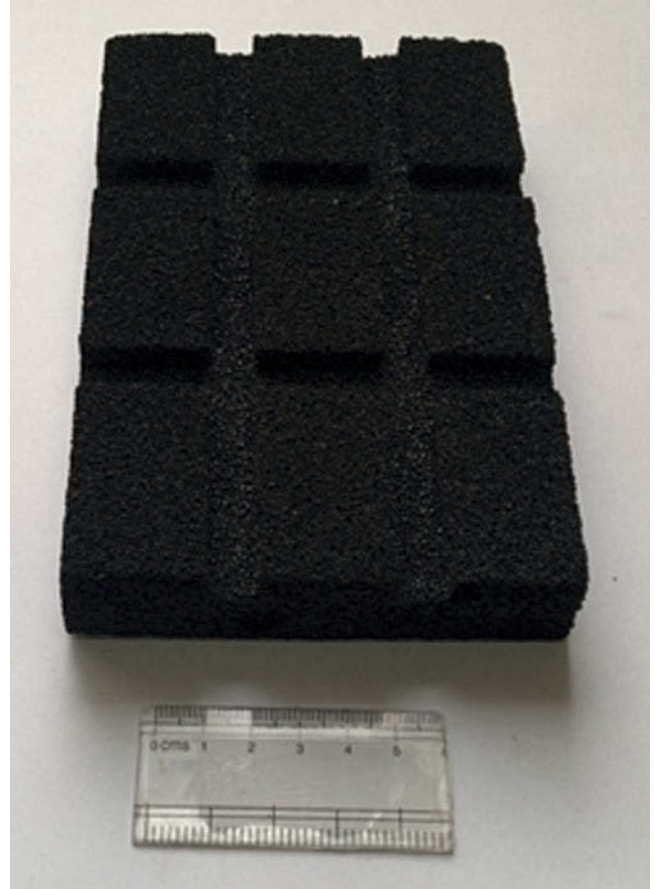
FIG. 9. Photograph showing slots made by milling a rectangular carbon bonded alumina foam body in a conventional milling machine using a high speed steel tool.
