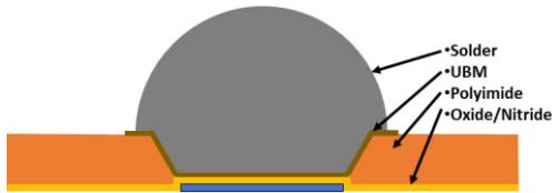
Figure 1: Standard C4 solder bump integration.
