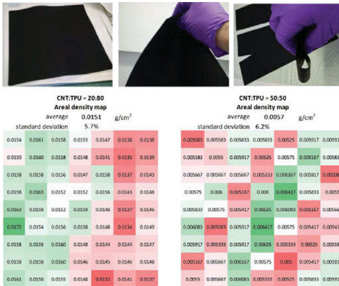
Figure 3. Larger scale, 30 cm x 30 cm, CNT-TPU fabrics. (Top) Photographs and (Bottom) areal density maps for fabrics with lower (20 wt.%) and higher (50 wt.%) CNT content.
