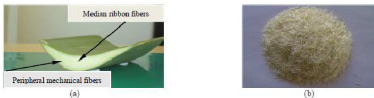
Figure 5. Sample of (a) cross-section of a fleshy, green sisal leaf showing fiber situation, (b) chopped sisal fibers.
