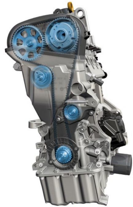
7 Timing drive of the 1.0-l three-cylinder engine
