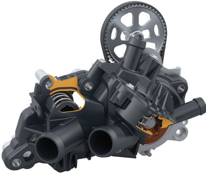
6 Water pump thermostat module with water circuit
