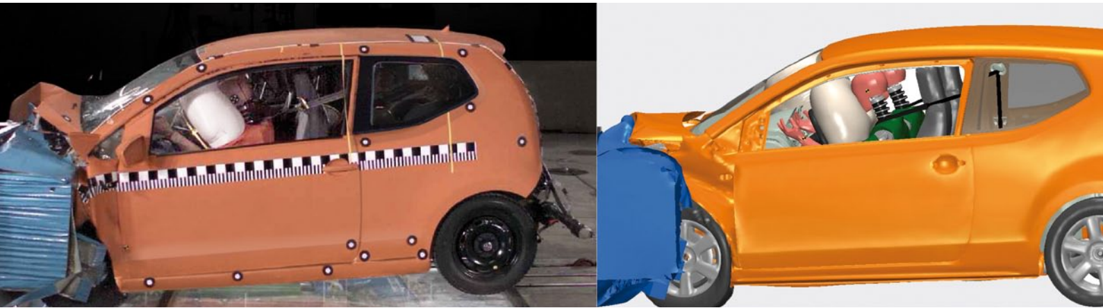
9 Frontal crash EuroNCAP; comparison test – simulation
