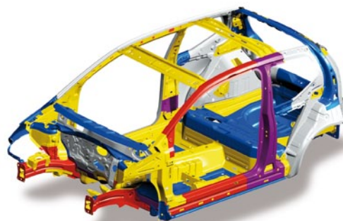
❶ Steel grade distribution in the body structure
