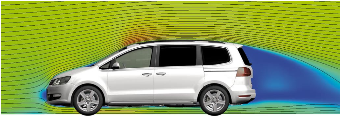
7 Calculation of airflow around the vehicle
