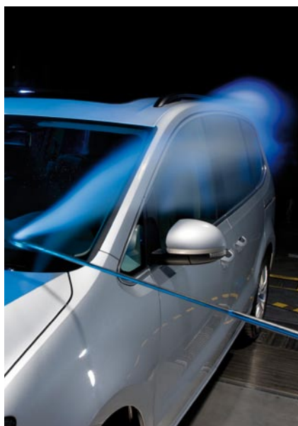
10 A-pillar with low-loss flow deflection
