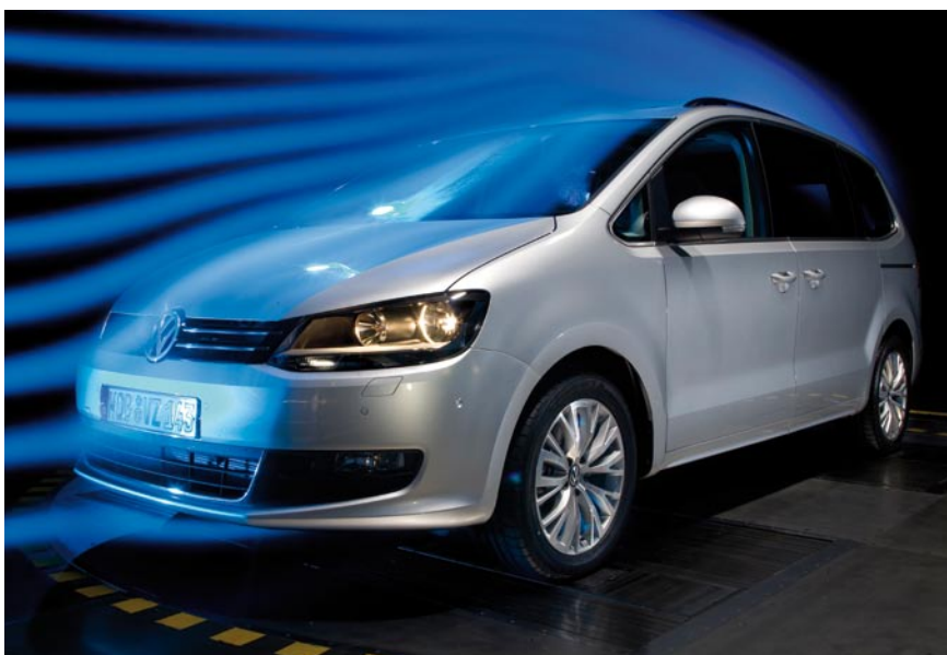
8 Measurement in the wind tunnel
