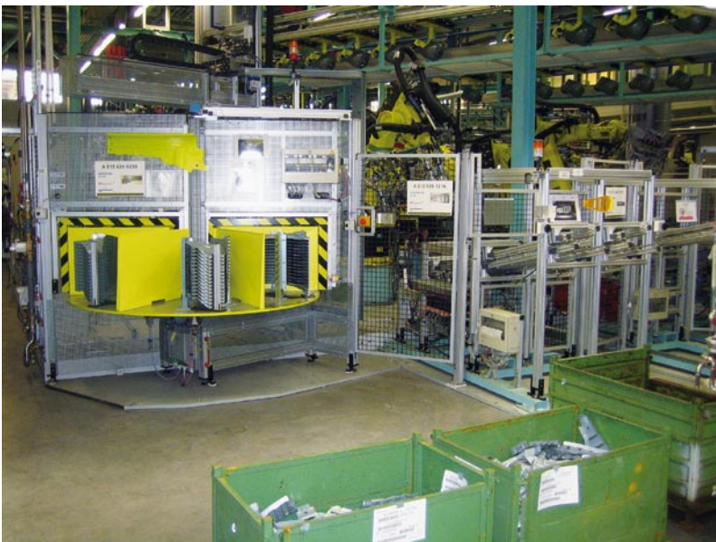
Figure 4: LCA (Low Cost Automation) type used in the E-Class
