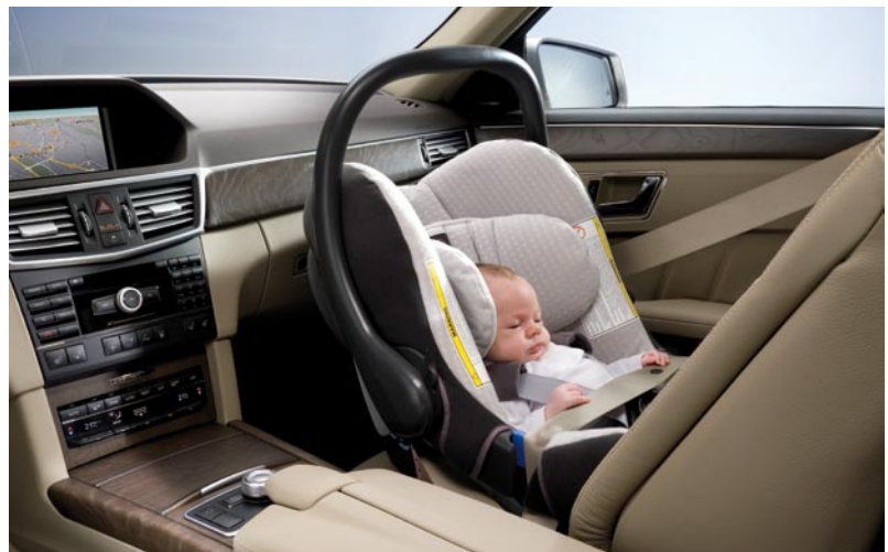
Figure 11: Child safety seat in front passengers position: Safety by the Automatic Child Seat Recognition System
