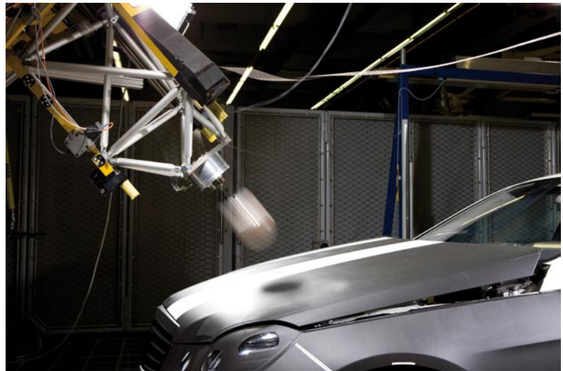
Figure 10: Excellent results in head impact testing for child and adult heads
