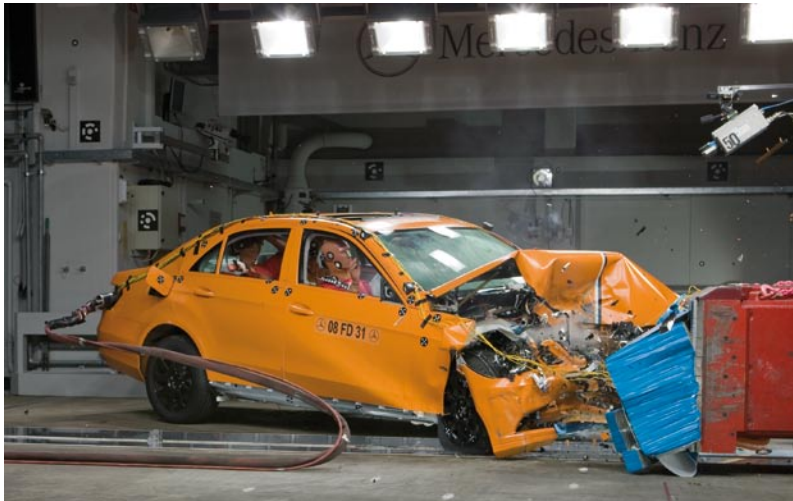
Figure 3: 40 % offset front crash
