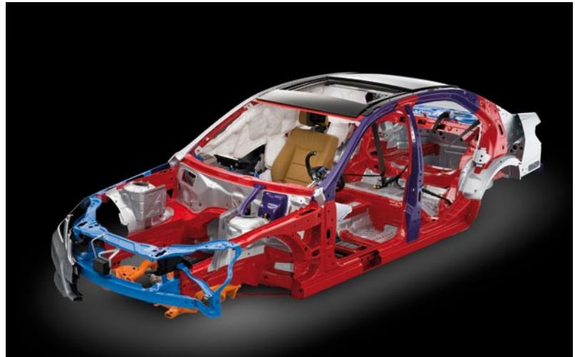
Figure 9: High and super high-strength steel used in the new E-Class body-in-white structure for more safety and fatigue strength
