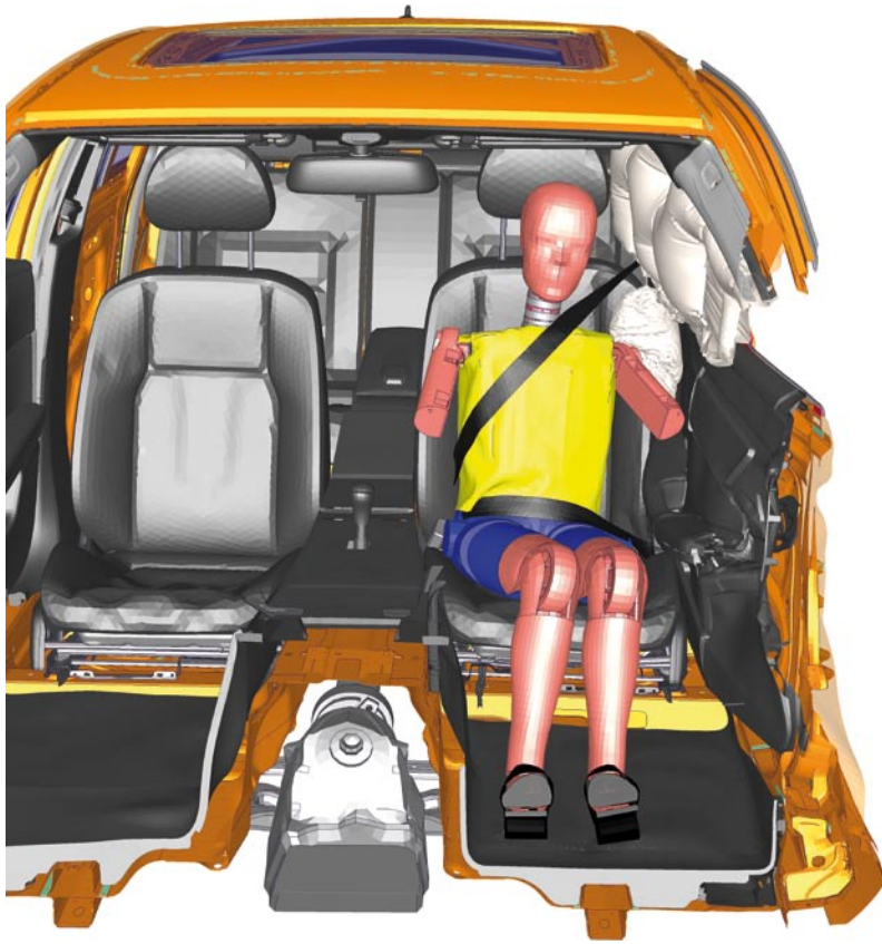
Figure 2: New E-Class numerical simulation of side collision
