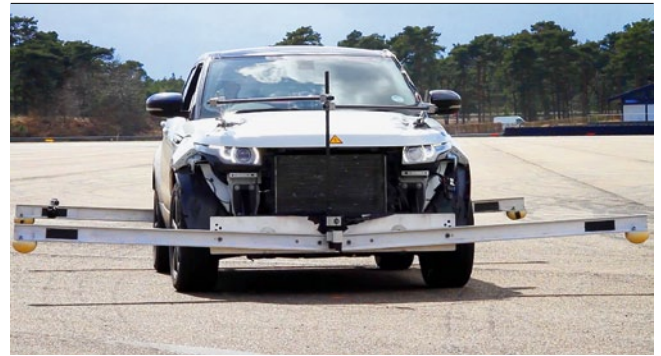
❶ Prototype with four individually driven wheels using the Range Rover Evoque
