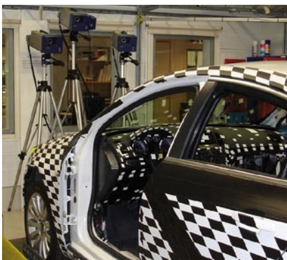
Figure 4: Modal correlation with 3D Scanning Vibrometer measurement points
