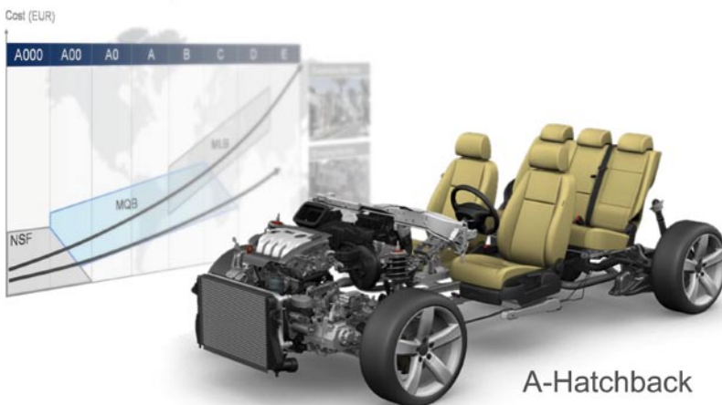
Figure 9: Basic concept of modular transverse matrix MQB
