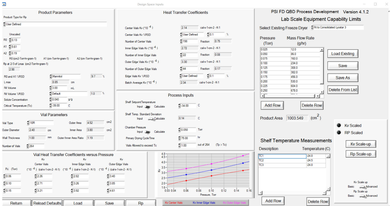
Fig. 2. Screen image of the lyophilization primary drying software model user input interface. Inputs include product, container, and lyophilizer equipment capability related parameters. Location- and pressure-dependent vial heat transfer coefficients as well as relative standard deviations for all parameters are required to describe contributors to drying heterogeneity and variation that will affect vial location dependent product temperatures and drying times
