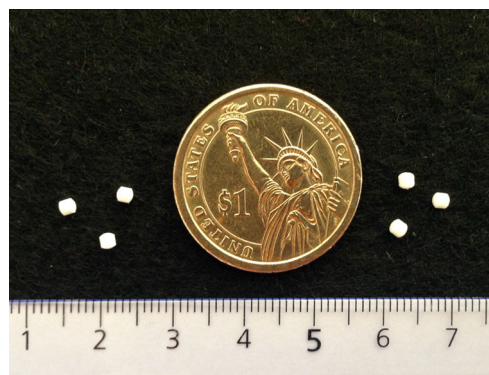
Fig. 1. Dimensions of uncoated mini-tablets ( left ) and coated mini-tablets ( right ) in relation to a 1 US dollar coin ( centre )
