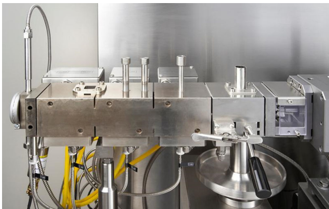
Fig. 20. Lab scale TSE with provision for probes for process monitoring
