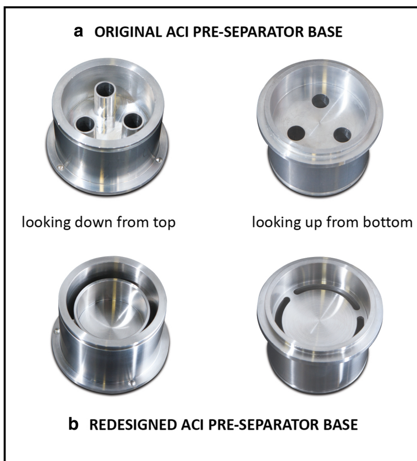
Fig. 1. Improvement by Roberts et al. (37) to the design of the base-plate of the Andersen cascade impactor. a The original design has three stand pipes oriented at 120°. b The stand-pipes are replaced by annular slits at the periphery of the base-plate in the redesign. Used with permission from Daryl Roberts
