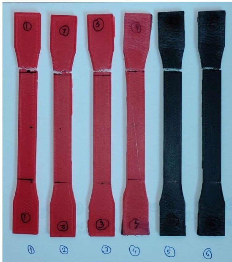
Fig. 9 Fractured 100% infill (line pattern)
