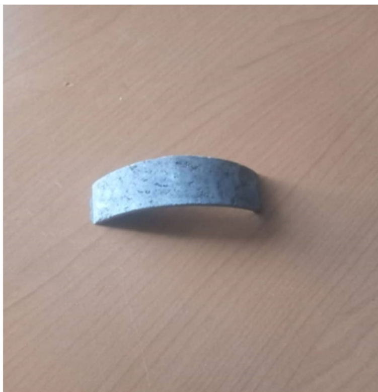
Fig. 7 Sample of the friction lining material developed
