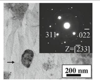
Fig. 6 TEM evidence showing the presence of Mg2Si in the fabricated composite sample [100]
