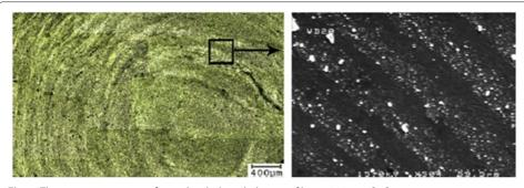
Fig. 5 The onion ring patterns formed with threaded pin profile at 1200 rpm [99]
