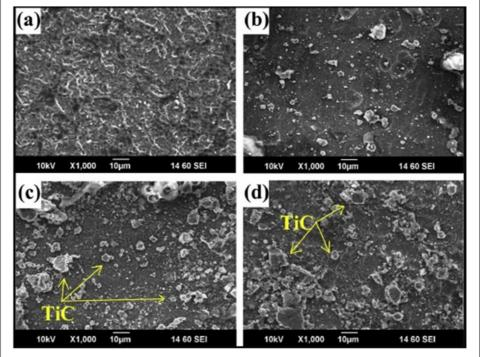
Fig. 10 SEM images of AZ31/TiC composite containing  $\bf a$  0 vol.% TiC,  $\bf b$  6 vol.% TiC,  $\bf c$  12 vol.% TiC, and  $\bf d$  18 vol.% TiC [112]
