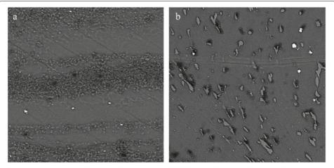
**Fig. 4** SEM images of friction stirred AZ91D/ $AI_2O_3$  processed at **a** RS= 800 rpm, TS = 40 mm/min, **b** RS = 800 rpm, TS = 80 mm/min [98]
