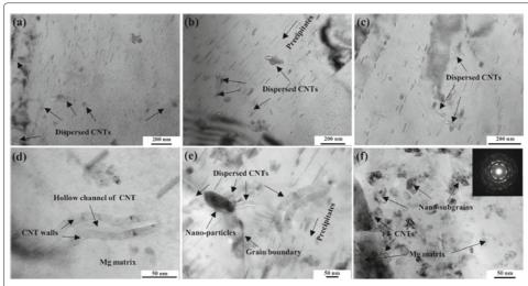
**Fig. 11** TEM images of FSPed Mg-CNT MMC: (**a–c**) Dispersion of CNTs, (**d, e**) CNTs morphology in MMC, (**f**) nano sub grains next to CNT [121]
