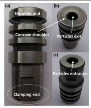
Fig. 12 Images of DFSP tool: a front view, b shoulder view, and c the clamping end [111]
