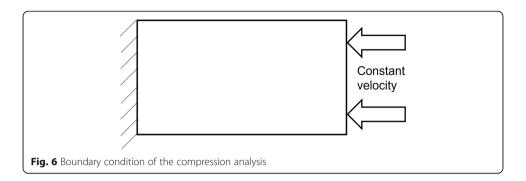
The boundary condition of the compression analysis is given in Fig. 6, the right side of the box is pushed to the left with constant velocity while the left side of the box is constrained in all direction. To illustrate the deformation of the box, the contour plot of the displacement of the box in the direction of the crash is given in Fig. 7. Figure 7 shows the contour plot of the displacement when the free side of the box is displaced 0.8004 m.
