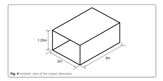
The damping factor, c, is assumed to be constant and it is computed from the loss material coefficient of Aluminum 6082-T6. We assume the loss material to be 0.05. Let  $\eta$  denote the loss material coefficient. Thus, the damping factor is as follows:
