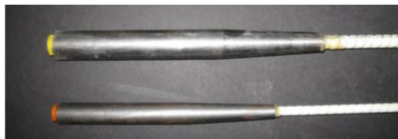
Fig. 2 Couplers used in tensile testing of GFRP bar specimens
