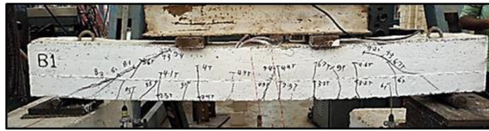
a: Crack Patterns at Failure load 9.80 ton for Tested Beam (B1)
