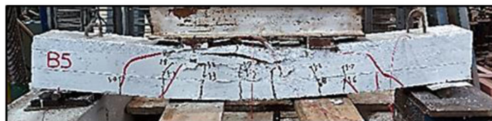
e: Crack Patterns at Failure load 32.40 ton for Tested Beam (B5)
