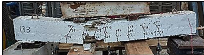
c: Crack Patterns at Failure load 39.2 ton for Tested Beam (B3)
