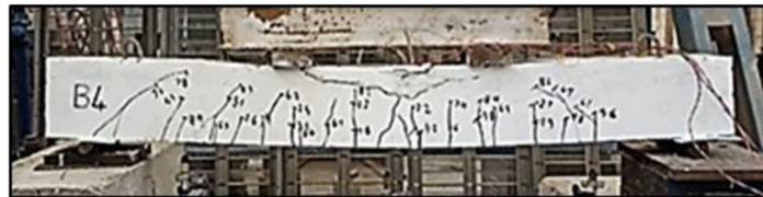
d: Crack Patterns at Failure load 23.93 ton for Tested Beam (B4)
