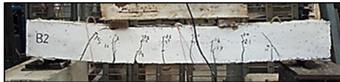
b: Crack Patterns at Failure load 33.90 ton for Tested Beam (B2)
