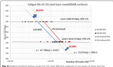
**Fig. 4** Rotating bending fatigue results for C45 steel (BM and surfaced) at two levels of stress and the confidence levels for each condition
