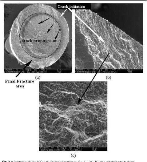
**Fig. 6 a** Fracture surfaces of C45 (S) fatigue specimen at N = 279,200. **b** Crack initiation site. **c** Mixed fracture modes: cleavage and dimple fracture
