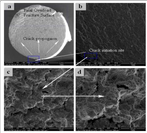
**Fig. 5 a** Fracture surfaces of C45 (BM) fatigue specimen at N = 133,500. **b** Crack initiation site. **c** Cleavage fracture. **d** Magnification of the initiation site
