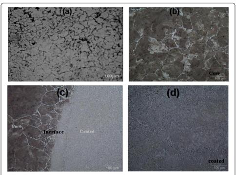
Fig. 2 a As-received C45 steel ferritic pearlitic microstructure. b Core microstructure, pearlite (black), and thin grain boundary ferrite (white). c Interface microstructure, Widmanstatten ferrite (surfaced) and pearlite, and thin grain boundary ferrite (core). d Surfaced microstructure Widmanstätten ferrite
