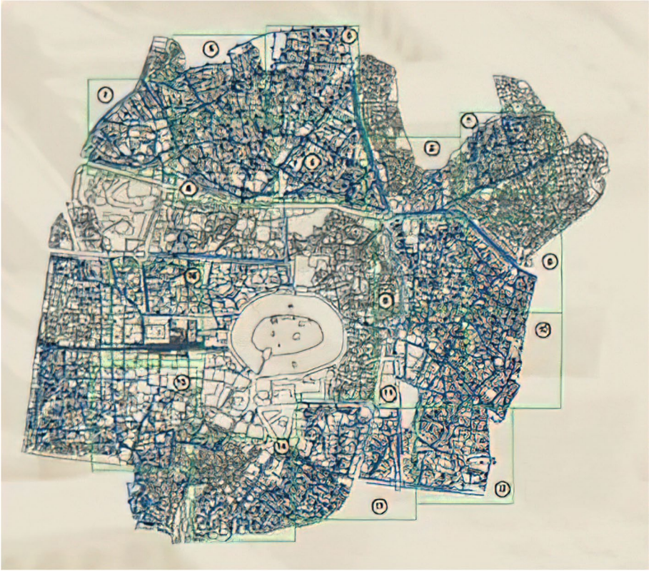
Fig. 11 Map Provided by the GTZ and DOCA on the Renewal of the Sewer and Drinking Water Networks in 2005 (Source: GTZ 2008)
