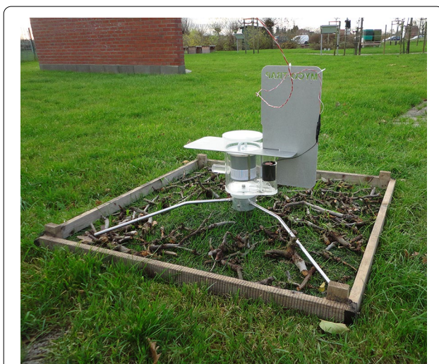
Fig. 2 Spore trap used for ascospore release studies in Northern Germany
