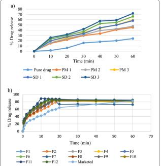
**Fig. 2** a Dissolution studies of PM and SD. The graph represents a comparative dissolution profile between pure drug, PM and SD. **b** Dissolution studies of marketed and formulated orodispersible tablets. The graph represents a comparative dissolution profile between the conventional marketed formulation and formulated orodispersible tablets
