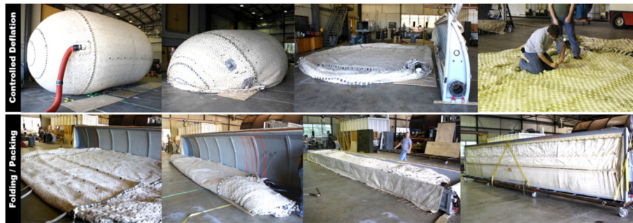
Fig. 9 Phase 2b-ET, full-scale testing, and three-layer Vectran plug. A sequence of controlled deflation, folding and packing into the soft-cover container [44, 69, 88]
