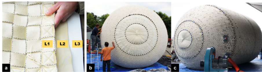
Fig. 6 Phase 2b. a Three-layer membrane configuration comprised of Vectran woven webbing (L1), protective Vectran fabric layer (L2), and inner bladder layer of urethane-coated polyester (L3). Unconfined inflation of (b) full-scale three-layer surrogate plug; (c) full-scale three-layer Vectran plug [44, 87, 88]
