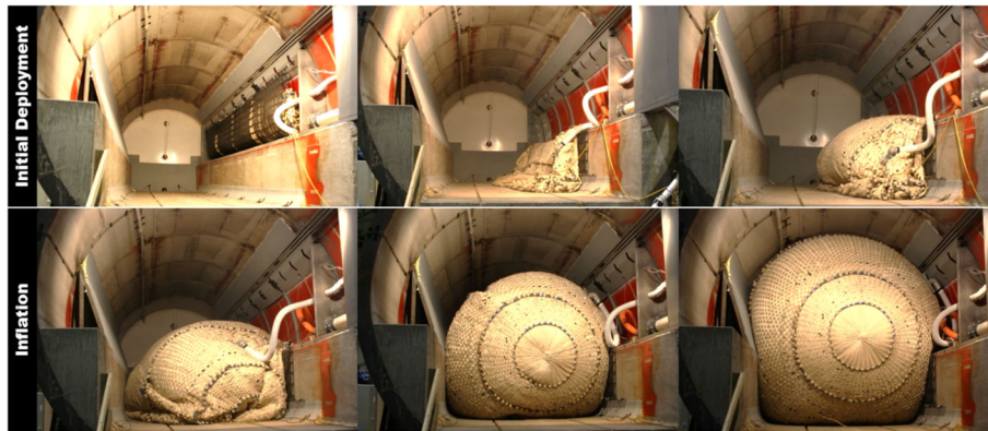
Fig. 8 Phase 2b, full-scale testing, and three-layer Vectran plug. Deployment and low-pressure air inflation for the initial positioning of the plug before flooding simulation [44, 88]
