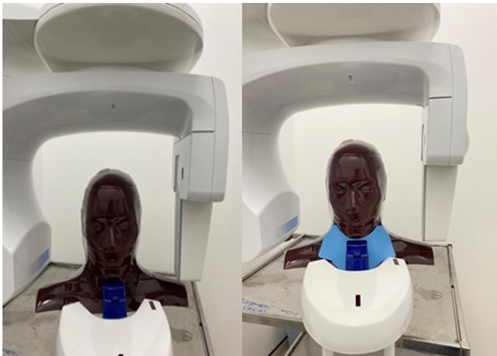
Fig. 1 The phantom setup for the dose reduction measurements. Without a thyroid shield (left), with a barium sulphate thyroid shield (right)
