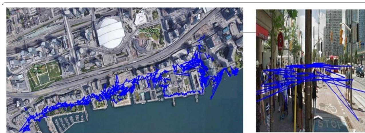
Fig. 1 GPS L1 code-only SPP solution for a kinematic dataset collected in a high multipath, urban environment
