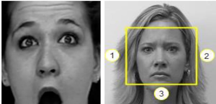
Fig. 6 Viola–Jones face detection with mouth missing (left): Border 3 must cover the whole mouth only, whereas Borders 1 and 2 must cover the face region (right)
