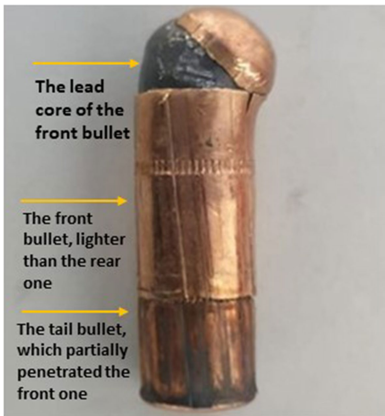
Fig. 1 The tandem bullets, merged together and extracted from the subject’s thigh. Note the chromatic difference between the front bullet and the back one, which is darker than the former
