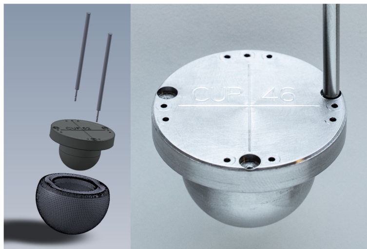
Fig. 2 A customised tool with a drill guide for inserting markers in the individual liner sizes of the system was developed (left) and machined in stainless steel (right). Three markers with increased depth ensured distinctive marker groups
