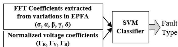
Fig. 10 Functional block diagram of SVM classifier for fault classification
