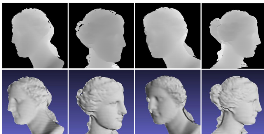
Fig. 19 Results of a plaster sculpture in different viewpoints. From top-to bottom: depth maps acquired by the proposed method and 3D reconstruction results
