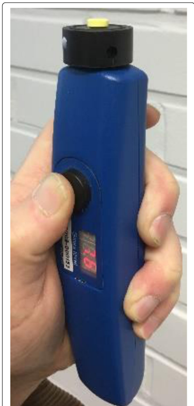
Fig. 1 A photo of the handheld glossmeter depicting how the measurement on the tablet samples were taken. The thumb is over the measurement button and the gloss reading is shown on the display
