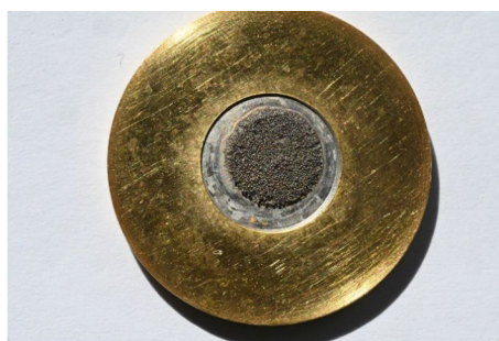
Fig. 6 Electrodeposited 70 mg ^{62}\text{Ni} ( 182\text{ mg/cm}^2 ) target onto a gold backing
