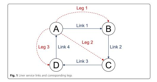
unloaded in Port C, which travel through Link 1 (A $\rightarrow$ B) and 2 (B $\rightarrow$ C). Since both links belong to the same liner service, the containers do not have to be transhipped at port B, which would have been the case otherwise.
