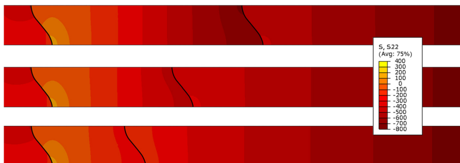
Fig. 6 Elastic stresses in 22-direction at the end of the heating step for three different thicknesses of bond coat and tbc
