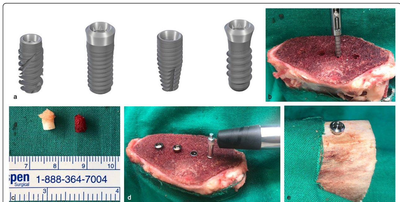
Fig. 1 a From left to right: BLX (4.0 × 10 mm), Straumann Tapered Effect (4.1 × 10 mm), Bone Level Tapered (4.1 × 10 mm), and Standard Plus (4.1 × 10 mm). (The figures were taken from the product catalogue with kind permission of Institute Straumann AG, Basel, Switzerland © AG, 2015. All rights reserved.) b The implants were inserted into the distal epiphysis on the longitudinal axis of the freshly slaughtered bovine ribs. The distance between the implant shoulders was set to a minimum of 5 mm. c Prior to implant placement, bone biopsies were taken to histologically examine the cortical bone height at the implant recipient area. Left: Biopsy taken from the control, right: Study group. d Measurement of the primary stability of the implants with Osstell device inserted in cancellous bone (from left to right, Straumann Tapered Effect [4,1 × 10 mm], Standard Plus [4,1 × 10 mm], Bone Level Tapered [4,1 × 10 mm], and BLX [4,0 × 10 mm]). e Implants were also individually inserted into the proximal diaphysis of the bovine ribs to serve as control. (Tapered Effect 4.1 × 10 mm)
