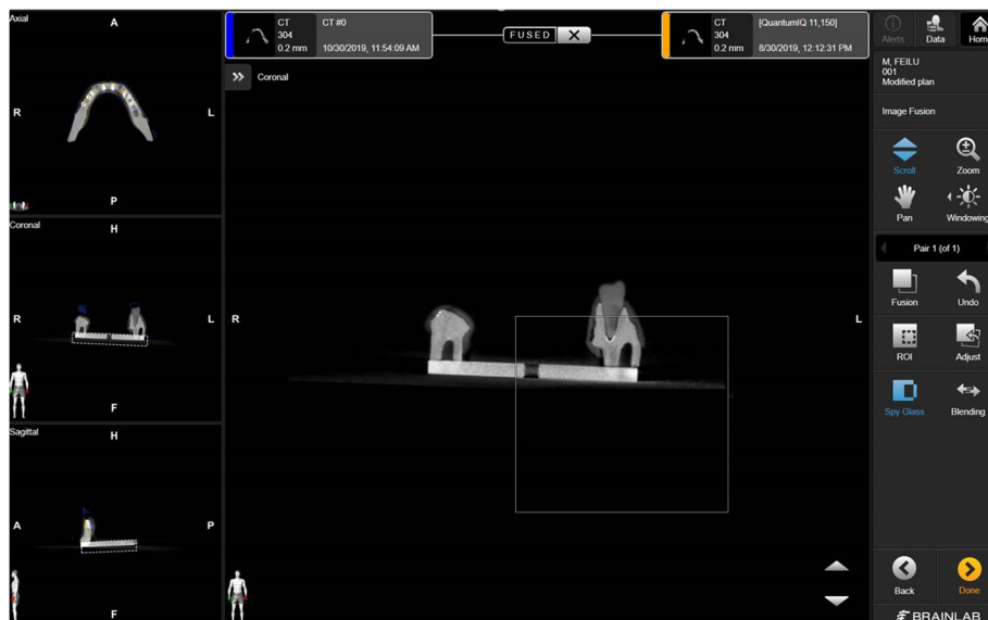
Fig. 7 CBCT images of test model and master model were fused based on the metal base
