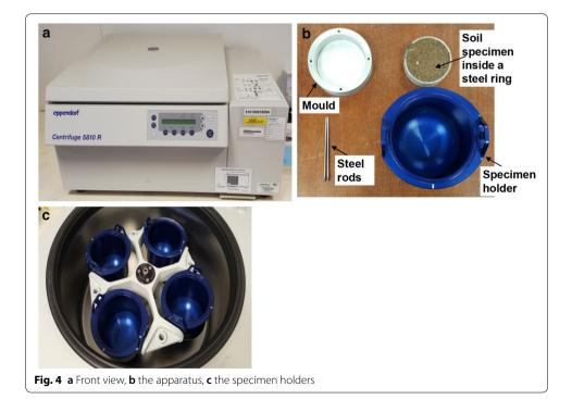
opposite sides to maintain the balance of the small-scale centrifuge machine (Fig. 4c). The test is performed at incremental angular velocities for specified durations. The angular velocities that are applied to the specimens varied from 200 rpm to 3900 rpm. The matric suction is calculated using Eq. 16.
