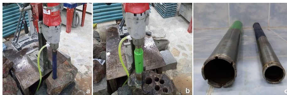
Fig. 1 Coring process by using drill bits with diameters of 32 mm (a) and 54 mm (b), different size core drillers (c)
