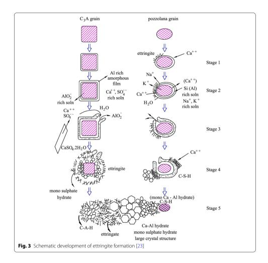
the broken film. Vacant space remains inside the film as the hydrates do not precipitate there because of high concentration of alkalies. For pozzolans with low alkalies, damage of amorphous Si, Al rich film enables Ca<sup>2+</sup> to travel into the inside of the film and precipitate calcium silicate and calcium aluminate hydrates on the surface of pozzolan grain. Therefore, no space is witnessed between pozzolan grains and hydrates.
