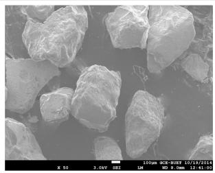
Fig. 2 Scanning electron microscopic view of sand particles
