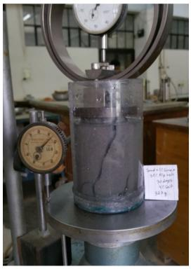
Fig. 5 Submerged specimen for unconfined compression test
