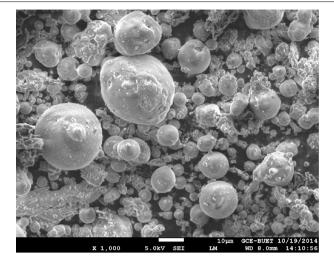
Fig. 3 Scanning electron microscopic view of fly ash particles
