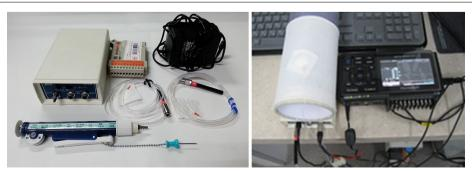
Fig. 2 AMI 3037-2-2B clothing pressure equipment (SANKO TSUSHO Co., Ltd. Japan)
