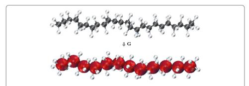
**Fig. 1** Representation of the AA-to-CG map G for polyethylene. Carbon atoms are shown in *gray*, hydrogen atoms are shown in *white*, and the CG particles are idealized by the *red spheres*
